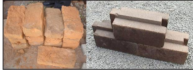
Fig 4: traditional fired brick      ISSB brick
