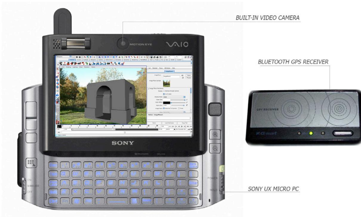
Figure 2: The ArchInSite Prototype, which utilizes a Sony UX Micro PC, GPS Receiver, and Maya Modeling Software
