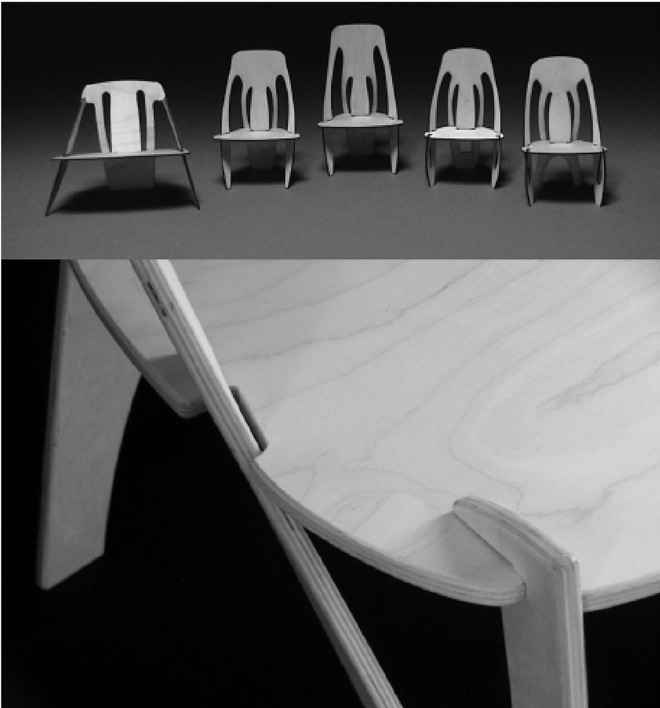
Figure 3. Wrap Chair - Scaled prototyping process (top) and detail of resulting leg joinery (bottom).
