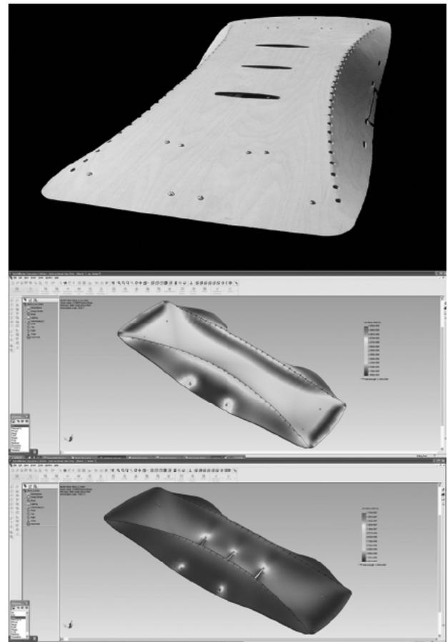
Figure 2. Petal Bench (top) with examples of digital stress analysis. No holes (middle) - Lighter tones indicate higher internal stresses. Adding holes (bottom) reduces stress and evens its distribution.
