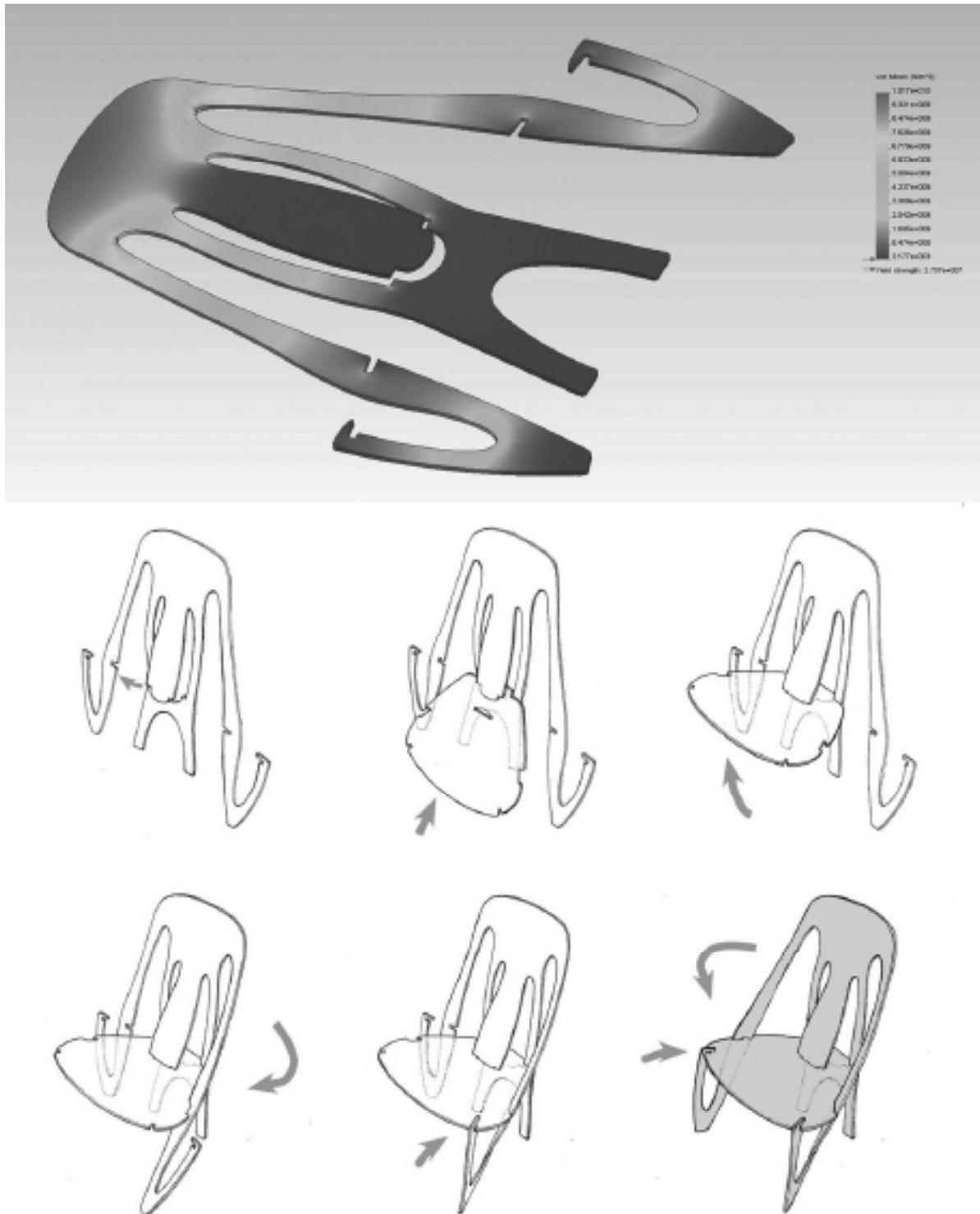
Figure 5. Wrap Chair -digital analysis of stress distribution directly contributes to the shape and formal language of the chair back (top) - Lighter tones indicate higher overall stresses. The assembly sequence (bottom) employs clip type joinery similar to that in the Clip Table's legs, and a wrapping joint type developed specifically for the structural needs of the chair's front legs.
