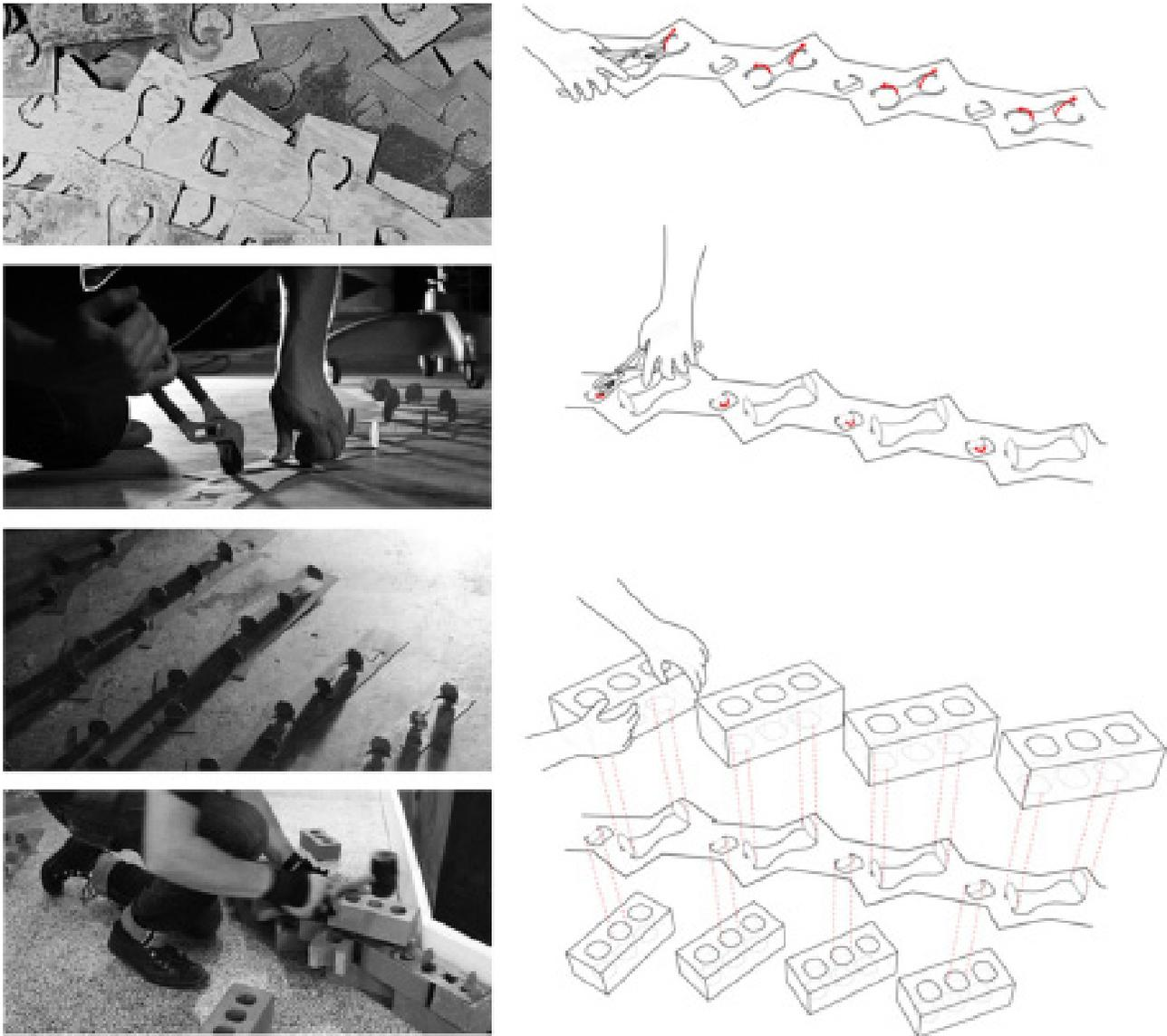
Figure 5: Diagrams and photos of Brick Veils jig and assembly sequence. (images: Cory Mattheis)
