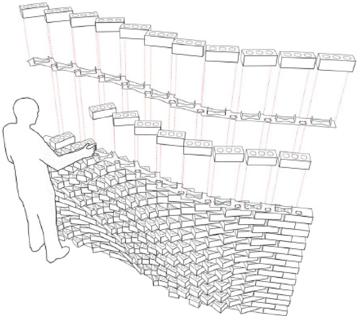
Figure 4: Diagram of Brick Veils system and assembly. (images: Cory Mattheis)
