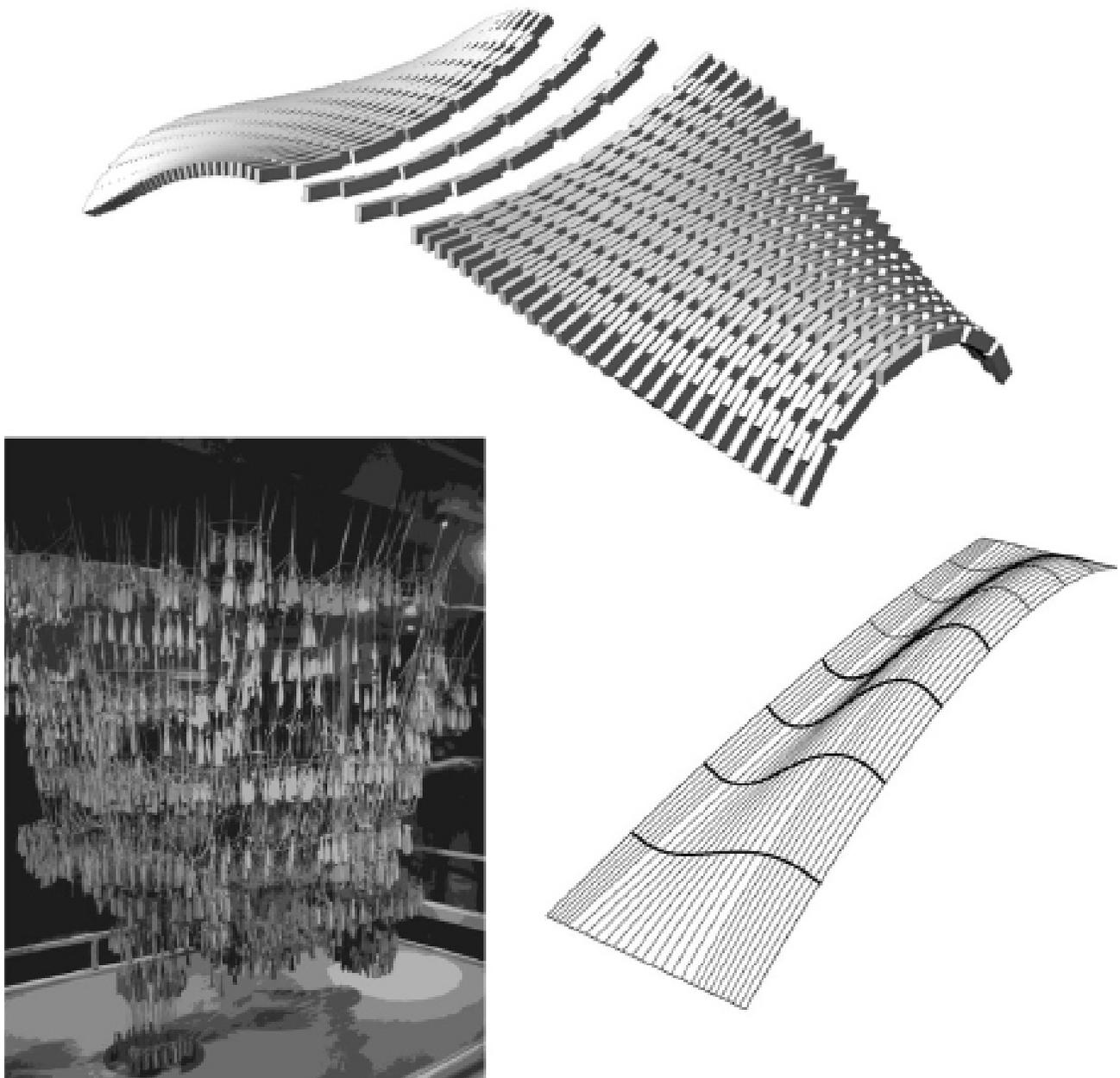
Figure 2: TOP: Scrapwood Shell design and construction concept diagram: curved courses are aggregated along a catenary path. BOTTOM: Structural form finding precedents. Left: Antonio Gaudi's hanging chain model of Sagrada Familia, Barcelona, ca. 1925. Right: Diagram of Eladio Dieste's 'gaussian' shells. (images: Rob Corser)
