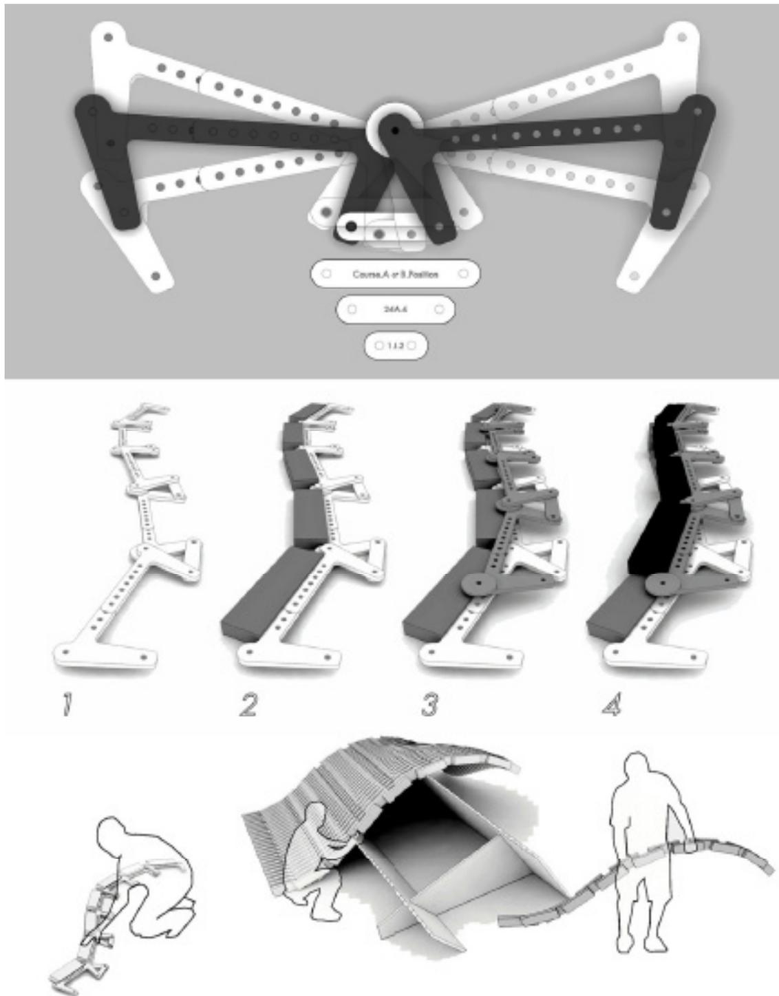
Figure 3: TOP: Diagram of the Jig shown in various positions. MIDDLE: Assembly of courses using adjustable jigs. 1. Bottom course jig is set with keys. 2. Wood blocks are set. 3. Upper course jig is placed and keys are set. 4. Upper layer blocks are glued and pneumatically nailed to bottom blocks. BOTTOM: Final shell assembly -courses are formed in jigs on left, and arranged on rail armature on the right. (images: Rob Corser and Scott Crawford)
