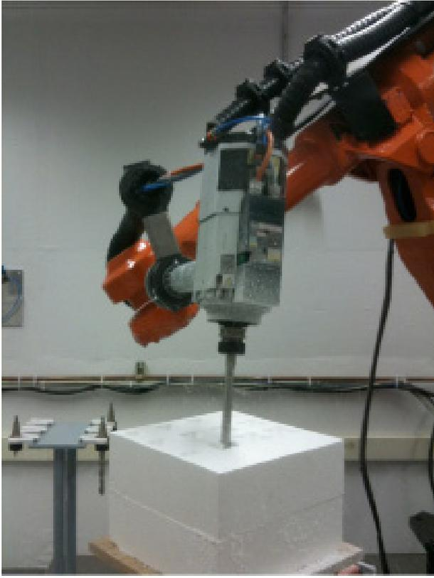
figure 2: industrial robot with milling tool
