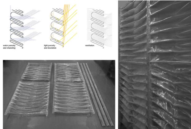
Figure 5. Vent Series performance parameters and composite panel assembly
