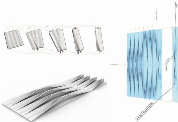
Figure 4. Jig configuration Diagram depicting the pattern of the draped textile and its pleated condition for gravity based panels
