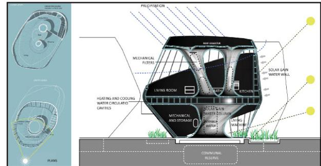
Figure 4: Unit hydrology and thermal heat gain systems
