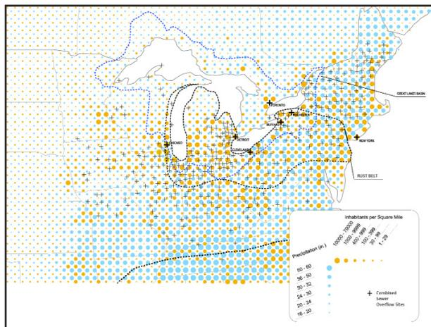
Figure 1: Precipitation and population in relation to combined storm and sewer system overflows in the eastern US
