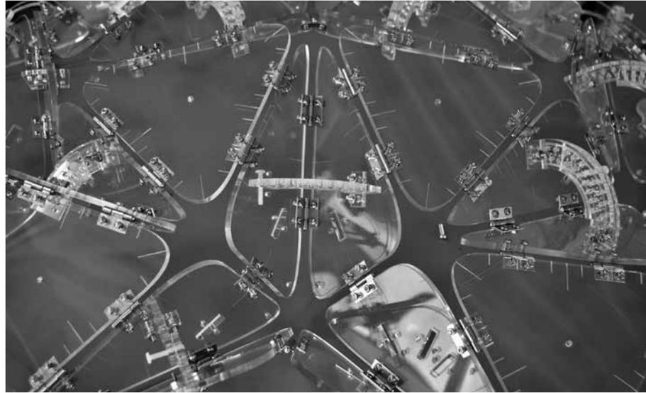
Prototype of folding tessellation using conventional hinges. Prototype uses 'protractors' to check angular movement
