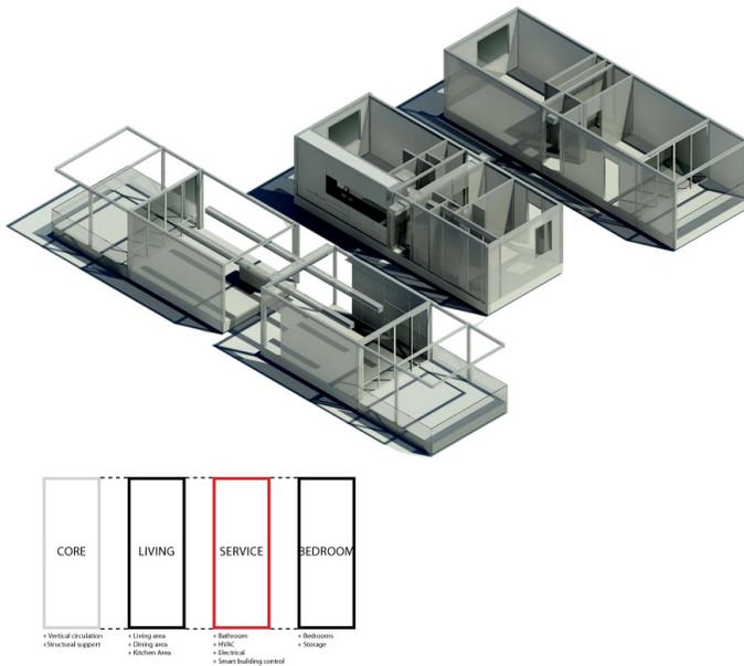
Figure 3. Three unit types make up a unit plan. The center unit is the “smart module” incorporating most of the building systems.
