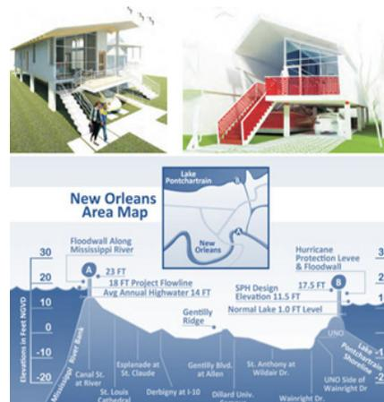
Figure 4: Emerging Green Builders South Florida Chapter Awards. Elevated, carbon-neutral houses (above) and section (below) of the city of New Orleans ground elevation from Canal St. at the Mississippi River to the Lakefront at U.N.O. by Katiuska Merino and Mabel Lanza, FIU, 2010.
