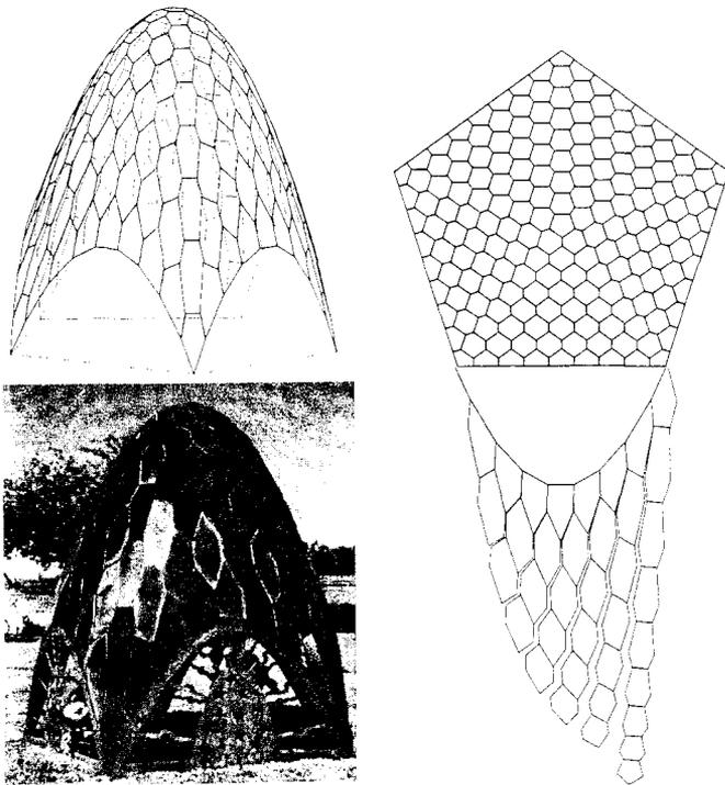
Figure 7: The ceramic dome Pentagonia, the computer model and the cutting pattern for the clay.
