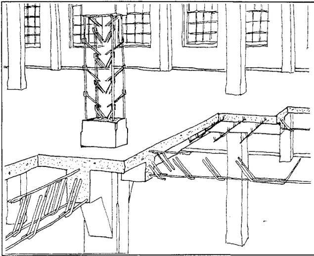
Figure 5. Kahn system of reinforced concrete, as used by Truscon, ca. 1904
