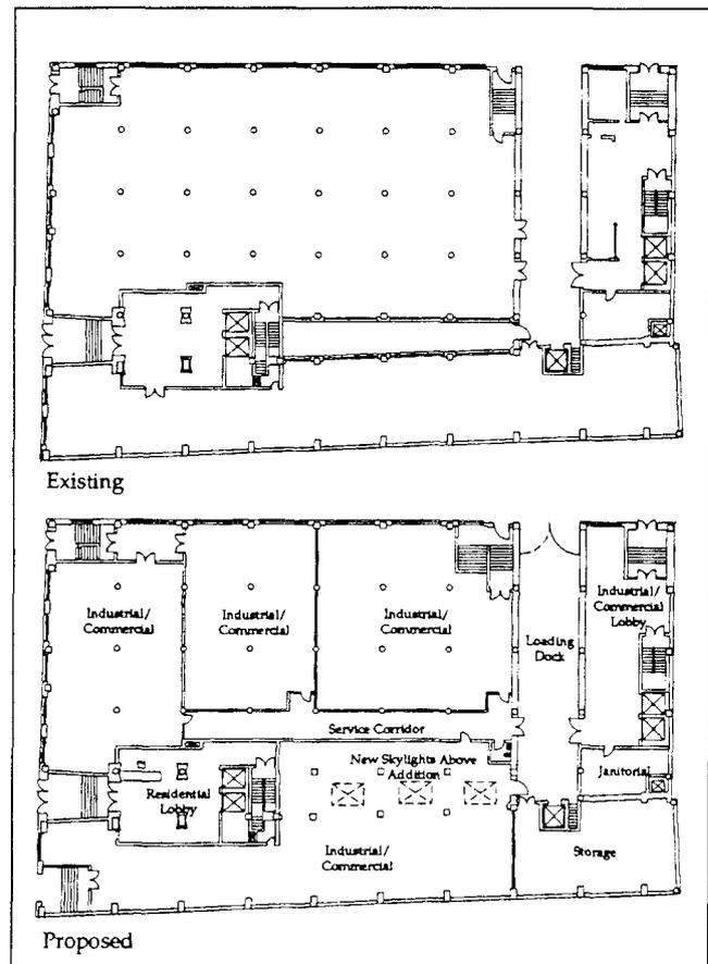
Figure 4: Ground Floor of Mayor Building—Existing (Top) and Proposed (Bottom) Plans
