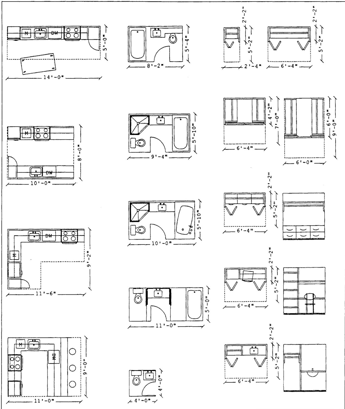
Figure 6: Kitchen, Bathroom and Storage Design Options
