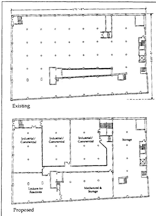
Fig. 3: Lower Level of Mayor Building—Existing (Top) and Proposed (Bottom) Plans
