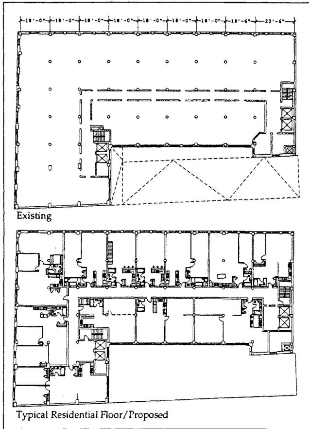
Figure 5: Upper Floor of Mayor Building—Existing (Top) and Proposed (Bottom) Plans for Typical Residential Floor
