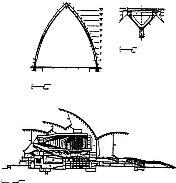
Fig. 3. a. Cross section through main shell rib segment and tile lid. b. Concert hall section. Taken from Philip Drew. Sydney Opera House. Jorn Utzon. London: Phaidon, 1995. p. 54, 59.
