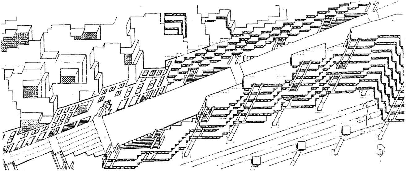
Fig. 4. Cutaway view showing coupled pan space frame and sloped street.
