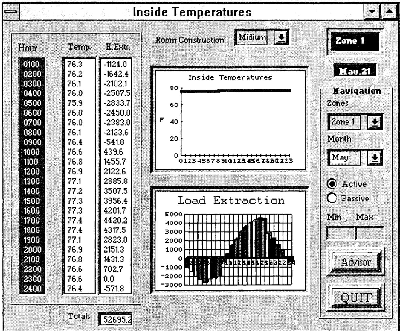
Fig. 5. The Hourly Temperature Analysis Screen
