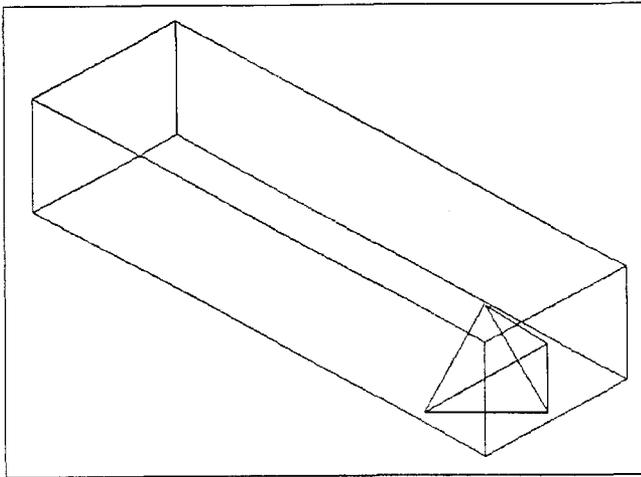
Fig. 5. The initial tetrahedral unit and boundary conditions.
