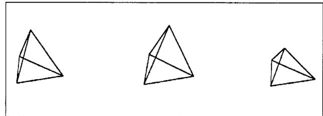
Fig. 3. A partial set of tetrahedral units available using a cuboctahedral nodal space frame system.
