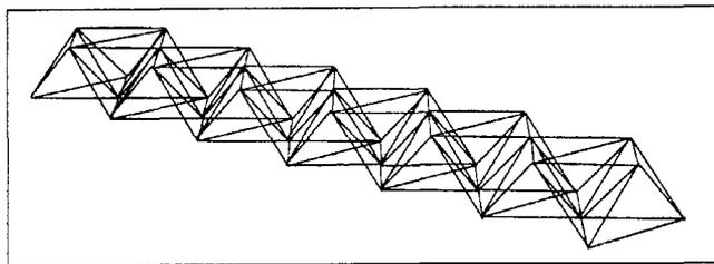
Fig. 7. A beam morphology generated by the grammar based computer program.
