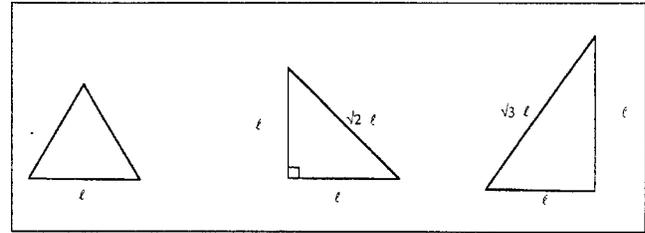
Fig. 2. A partial set of triangular faces available using a cuboctahedral nodal space frame system.
