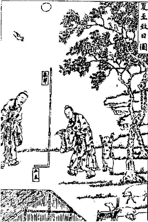
Fig. 5. The ancient Chinese found that the sun cast the shortest shadow of the pole to the north and south.
