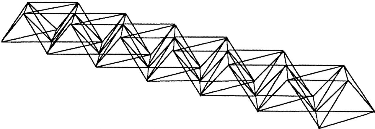
Figure 7. A beam morphology generated by the grammar based computer program.
