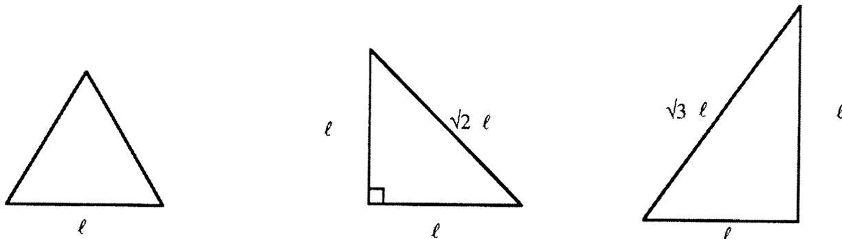
Figure 2. A partial set of triangular faces available using a cuboctahedral nodal space frame system.
