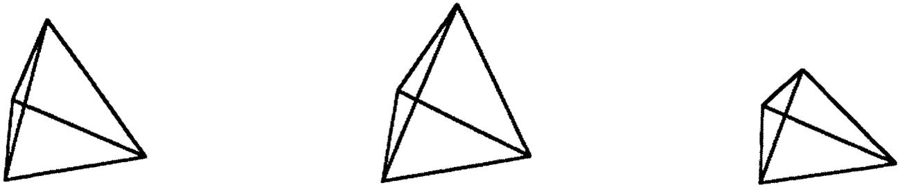
Figure 3. A partial set of tetrahedral units available using a cuboctahedral nodal space frame system.
