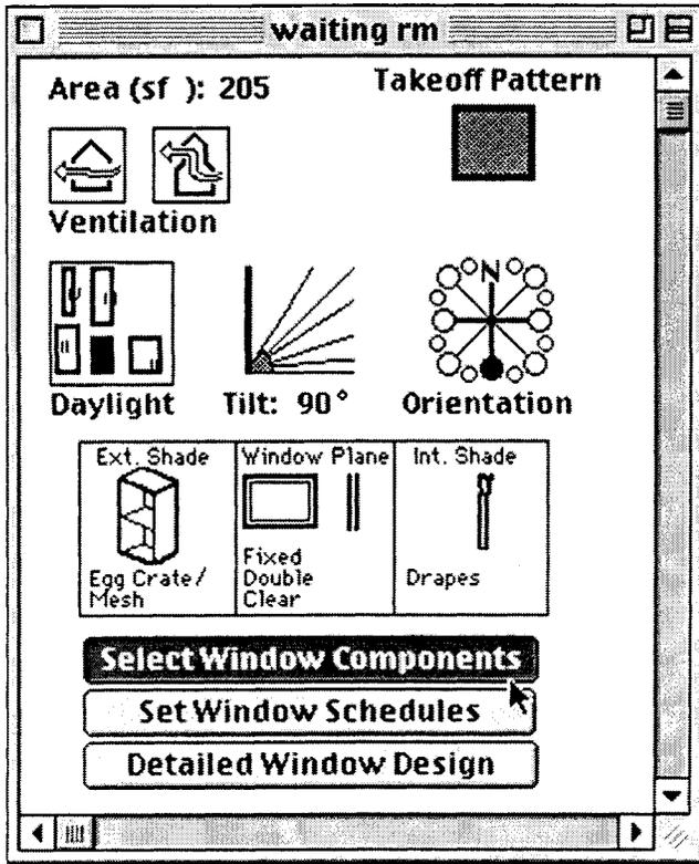
Fig. 8 Example of Specification for Windows
