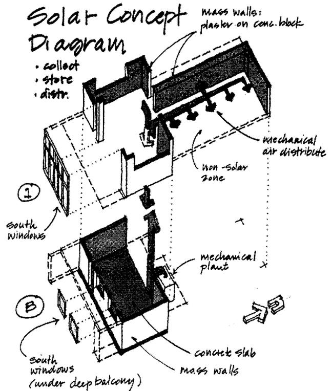
Fig 5 Example of Diagrams for Building's Solar Concept
