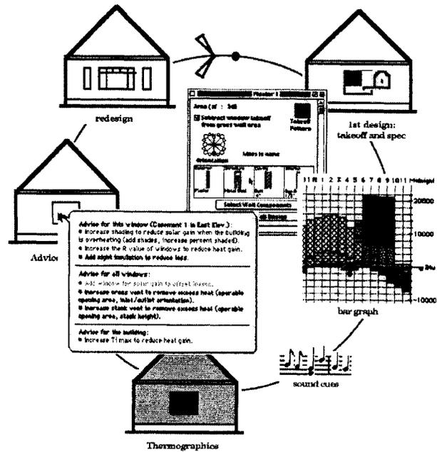
Figure 2: The design process using *Energy Scheming*.
