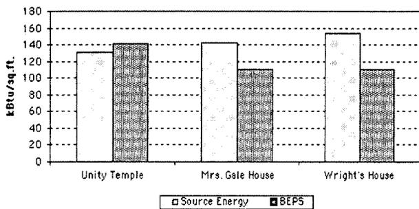
Fig. 5. A comparison of the Source Energy of each building with BEPS
