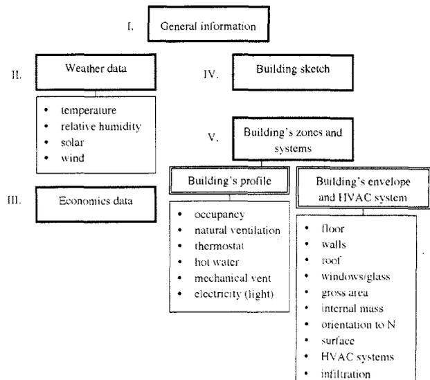
Fig. 4. A schematic structure of an input file
