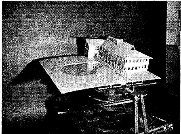
Fig. 4. View of model on heliodon.
