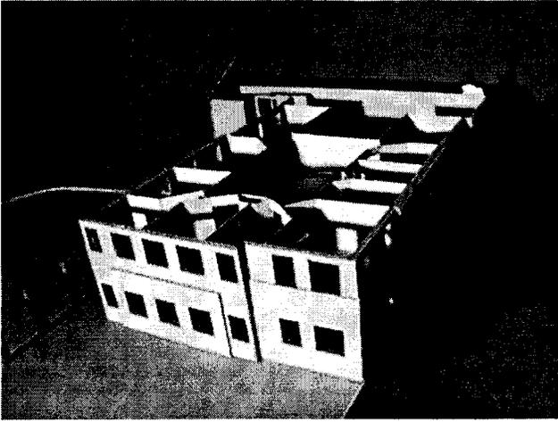
Fig. 6. View of model on heliodon with roof removed to show interior partitioning
