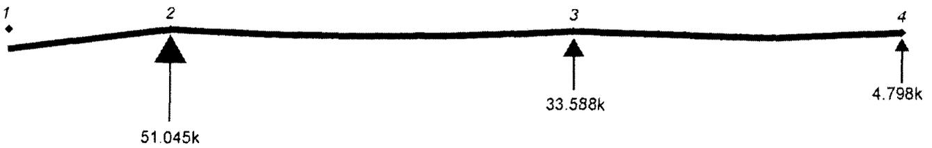
Fig. IV Reactions for continuous beam (prestressed concrete solution, west cantilevered element).
