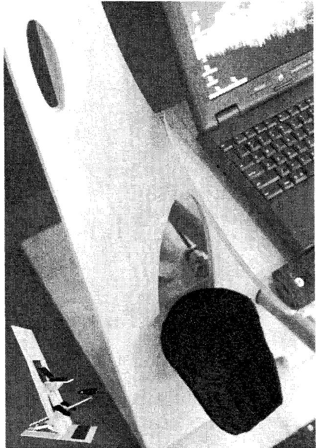
Fig. 1. The actuated knee-rest and tray of the Laptop Easel (patent pending)
