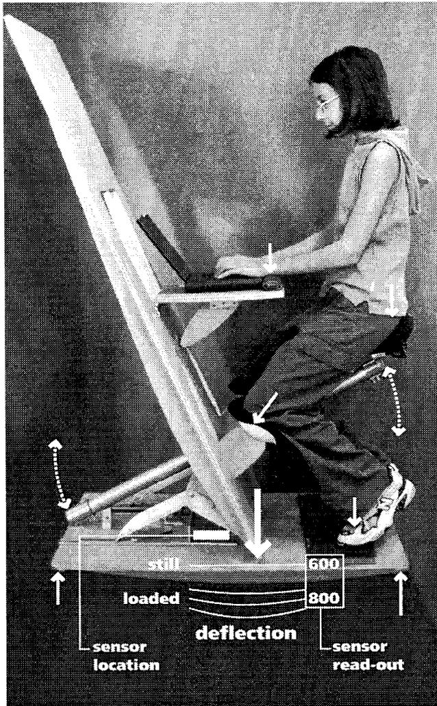
Fig. 6. Bending and actuation vectors of the Laptop Easel
