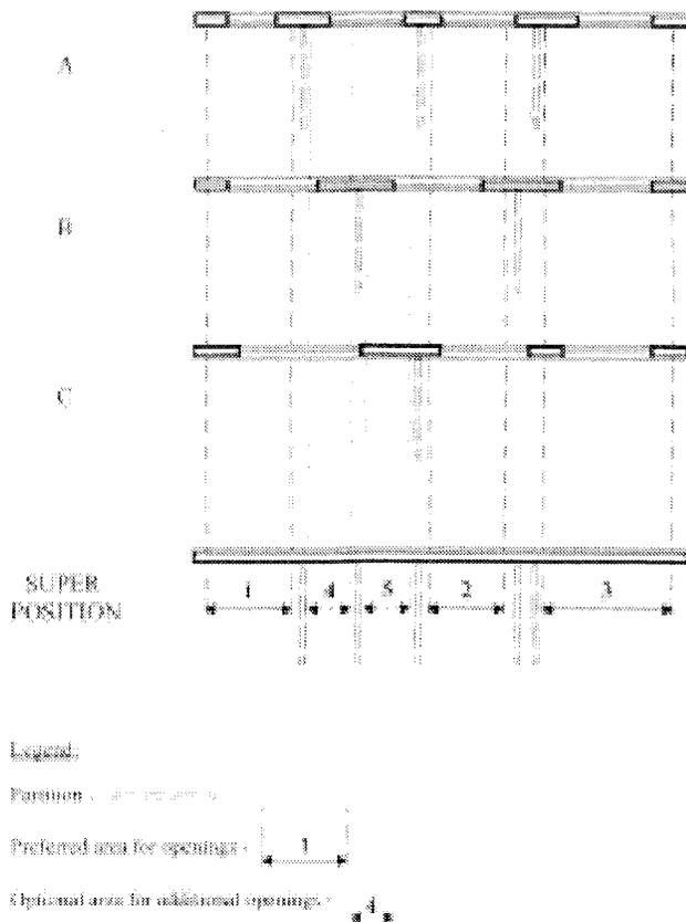
Fig. 5. Finding appropriate location for openings in facades - superposition of three floor plan alternatives
