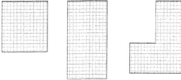
Fig. 1. Square, rectangular and 'L shaped' floor plans
