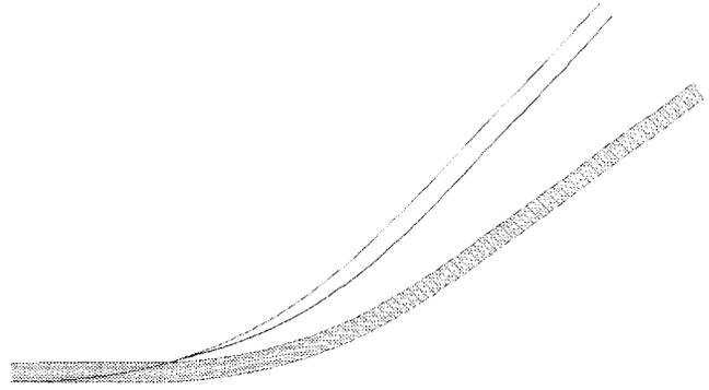
Figure 6. The edges of the base layer in the torsioned beam and developed in the plane.
