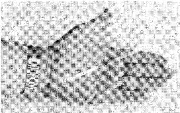
Figure 4. A radio frequency identification transponder.
