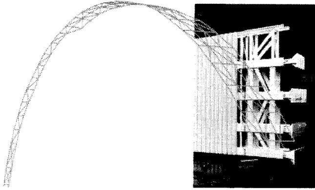
Figure 3. CNC bending of T beams, Courmayeur Tunnel.
