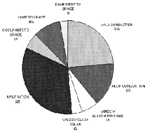
Figure 8 - Total building peak load components (kBtu/h)
