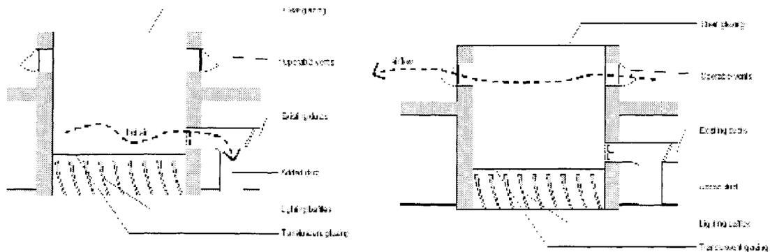
Figure 11 - Sections of skylight in winter (left) and summer (right)
