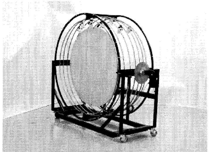
FIG. 4 The Sun Emulator in its storage mode. The cradle with the 7 hoops is set for 0 latitude, as it would be to simulate the solar geometry at the equator.
