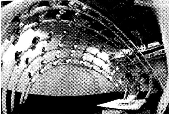
FIG. 2 This type of heliodon uses multiple lamps to simulate the daily and annual motion of the sun. For latitude adjustment the model table can be tilted a maximum of 10 degrees each way.
