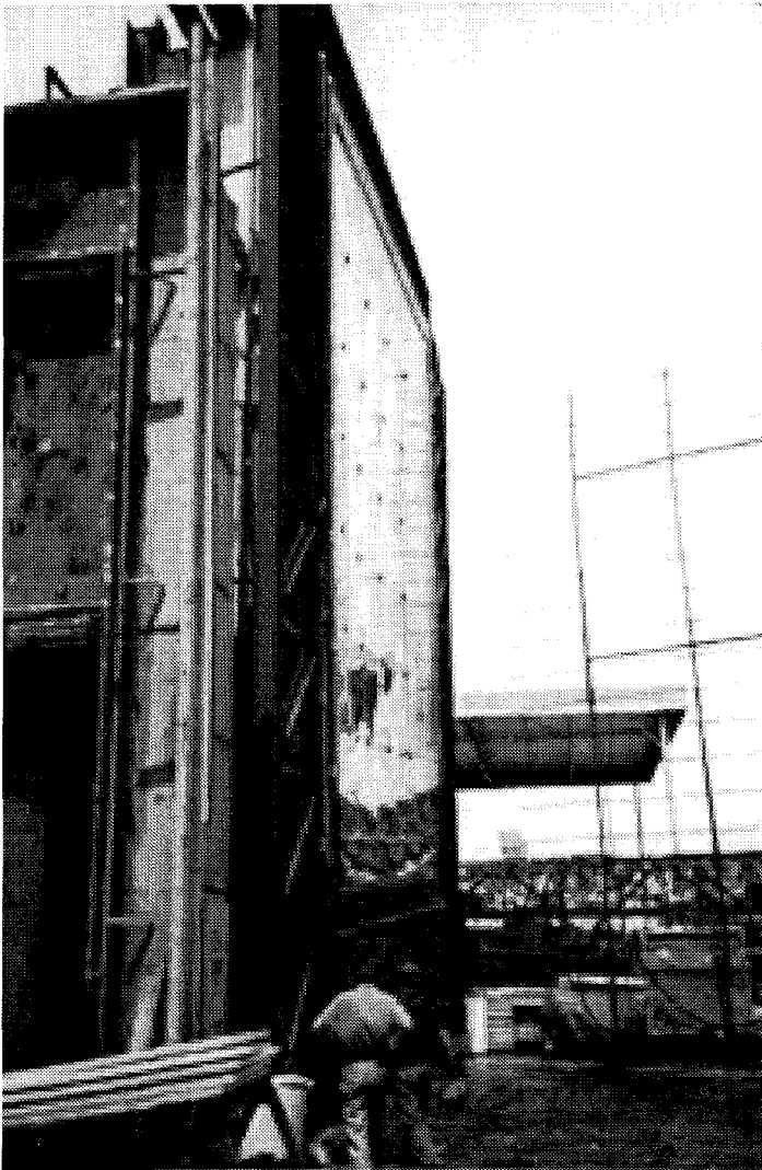
Figure 7: Test specimen exhibiting large deflections without failure (courtesy of ASI)
