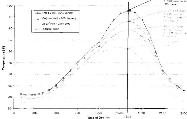
Fig. 2. Predicted Façade Zone Temperatures at 11th Floor (varying vent opening size)
