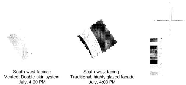
Fig. 5. Comparison of Predicted Thermal Comfort Adjacent to Different Façade Systems
