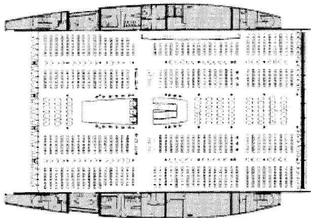
Fig. 2. The Phoenix Central Library: 5<sup>th</sup> floor plan with flanking saddlebags on the east and west sides of the main reading room.
