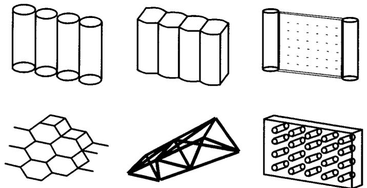
Fig. 2. RPC: Potential structural systems
