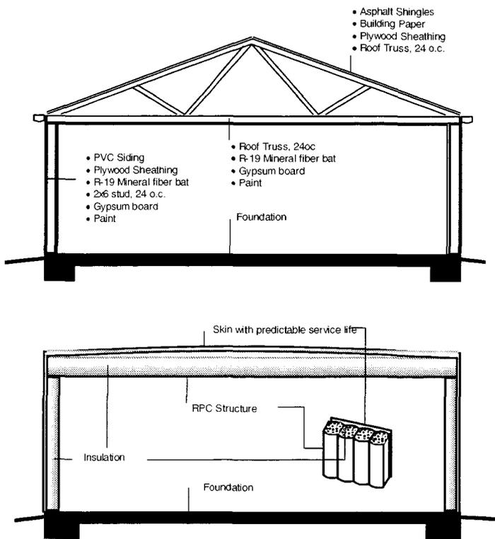
Fig. 3. Sections through WLF and RPC systems
