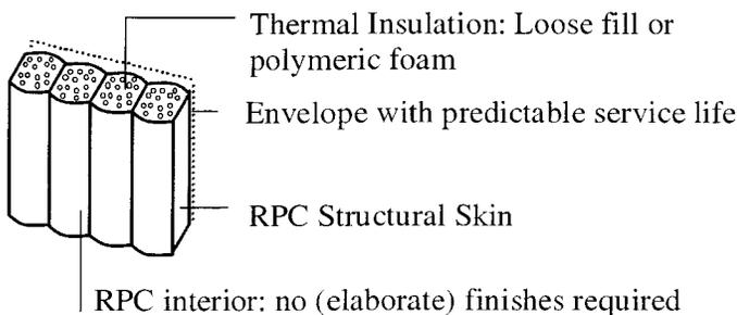
Fig. 4. Composition of the RPC wall/roof assembly used in our case study
