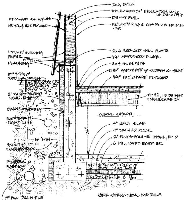
Fig.2. Wall and foundation construction section
