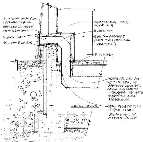
Fig. 3. Crawl space ventilation detail.
