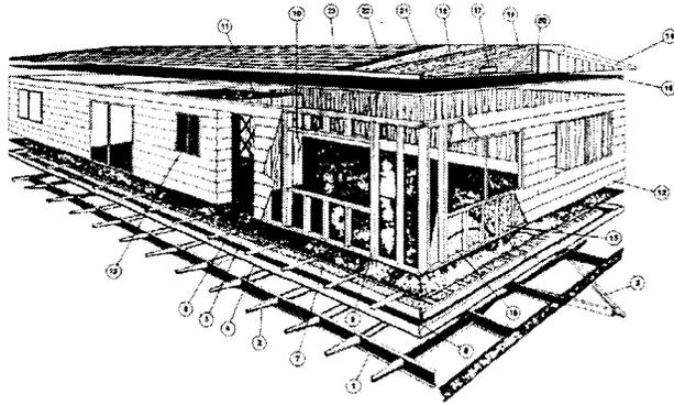
*Fig. 1. A typical current configuration of multiple separated components within a standard manufactured house.*
