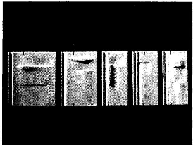
Fig. 6. Milled panel formwork at 1/4" scale.
