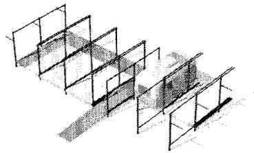
Fig. 4: Fly-foam floor foundation with bamboo flooring inside the structure, and bio-composite choice deck outside the structure.
