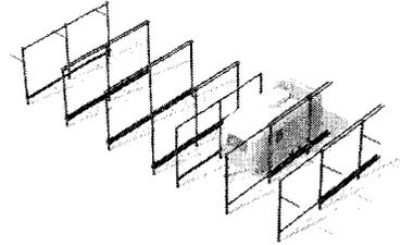
Fig. 3: Airstream Trailer as Mobile Utility Unit with B-Line structural columns and Beams
