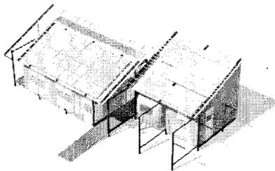
Fig. 6: Solar PV panels on metal roofing deck with Hardie board over Structural Insulated Panels for wall infill.
