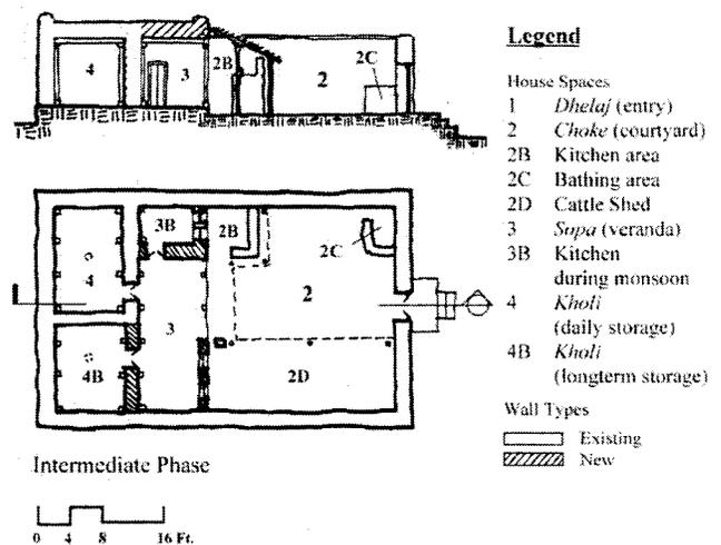
Fig. 2. Section and plan of a typical wada style house.
