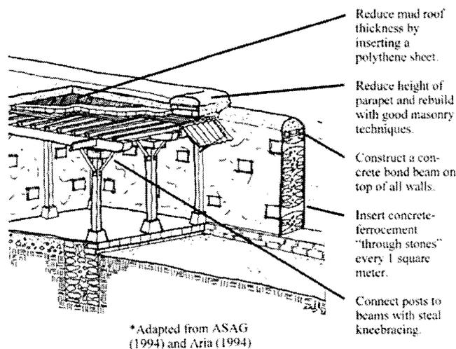
Fig. 6. Retrofitting modifications to vernacular wada style housing, developed by Dr. Aria (1994) and Rajendra Desai, formerly of ASAG (1994).
