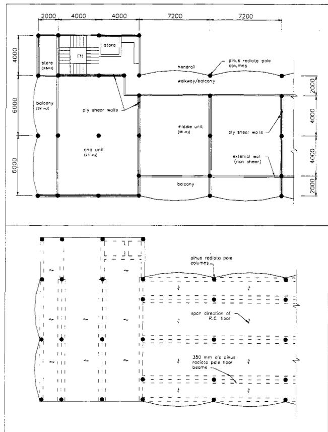
Fig. 1. Prototype Pole Building - above, plan of units; below, plan of main structure.
