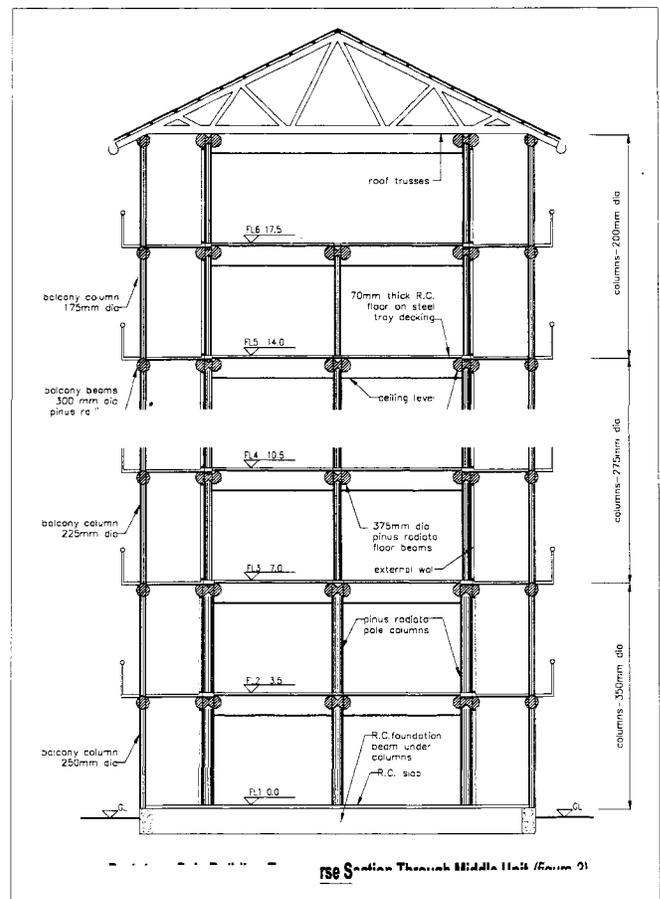
Fig. 2. Prototype Pole Building - transverse section through middle unit.
